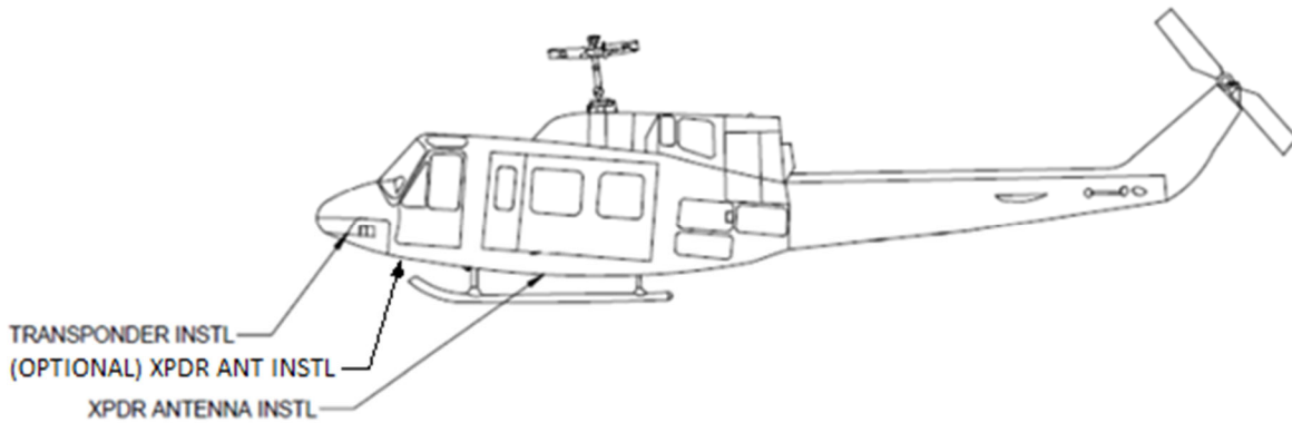
Figure 97-2 – Transponder System Location
